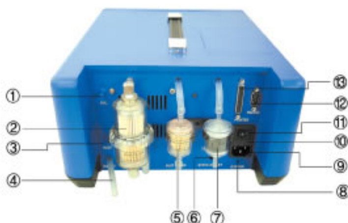
1. Calibration inlet 2. Main Filter 3. Inlet 4. Out let 5. Dust Filter 6. Extra Outlet 7. Zero Filter 8. Ground 9. Power Soket 10. Fuse Box 11. Power Switch 12. RS232 Port 13. Printer Port
